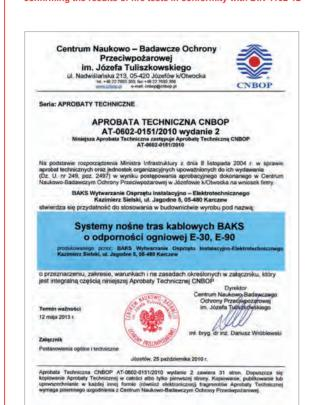
This certificate confirms that Support Systems of Cable Runways from BAKS, Integrated Function Maintenance Rated Rated E30, E90 are fully compliant to the DIN 4102-12 standard, based upon fire tests conducted in accredited testing centres.
