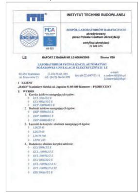
Testing laboratory of the Building Research Institute in Poland (ITB) decided upon testing of fully assembled cable trays and ladders from BAKS that the above products fully comply with the PN-IEC 61537:2003 (U) standard in respect of electrical properties of maintaining system circuit integrity. Mechanical connections of cable tray and ladder lengths allows for equipotential bonding for electrical continuity in accordance with the requirements of this standard.
